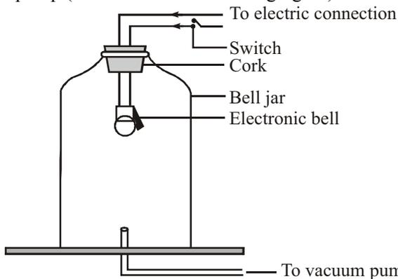
Initially, one can hear the sound of the ringing bell. Now, pump out some air from the bell jar using the vacuum pump. It will be observed that the sound
